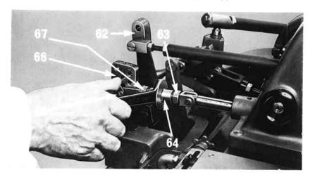
e) Lock the nuts (67) and (63), taking care to ensure that the flat on the jet block driving rod (80) remains in the horizontal position – and then check the setting once again.
