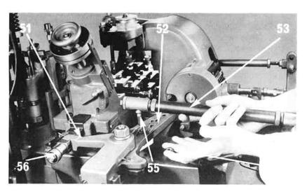
not already disconnected) by removing the nut (54) which secures the connecting tube ball end joint (55) to the intermediate lever.
