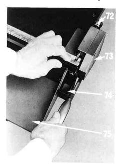
40.22 Removing the mould from the machine
