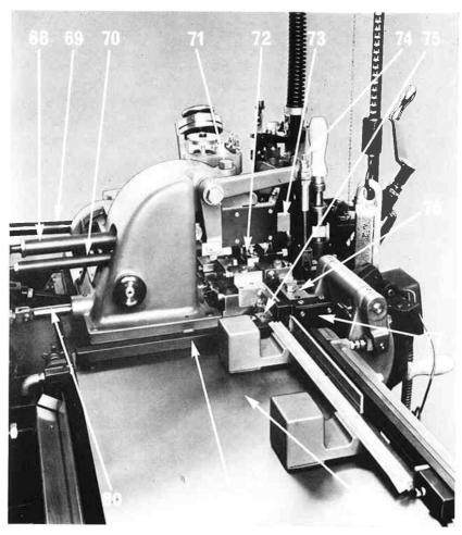
mould blade stop lever handle is in the position marked 'Leads'. Turn on the water supply; check the flow at the water supply tap and adjust as necessary.
