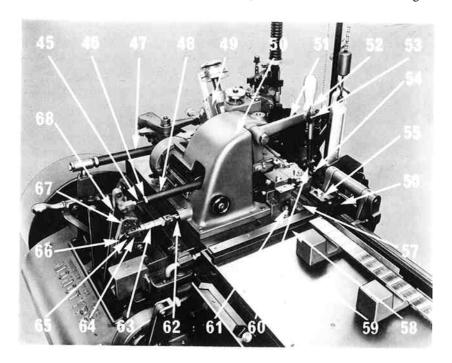
When the above adjustment is correctly made, the jet block driving rod, connecting rod yoke position pin will be correct for all sizes cast on the strip moulds, if it is placed in the 12pt hole in the type carrier cam lever extension.
